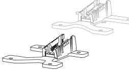
Module stops and screw connection 35 mm
